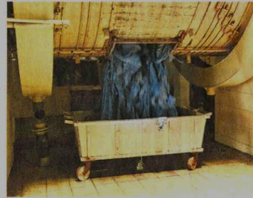
Leather mixed with waste water containing chromium, salt and acid comes out of the mixing drum under the traditional process; (right) leather produced with the WCTT process BIJOY GHOSH
