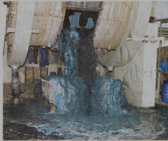
Leather mixed with waste water containing chromium, salt and acid comes out of the mixing drum under the traditional process; (right) leather produced with the WCTT process BIJOY GHOSH
